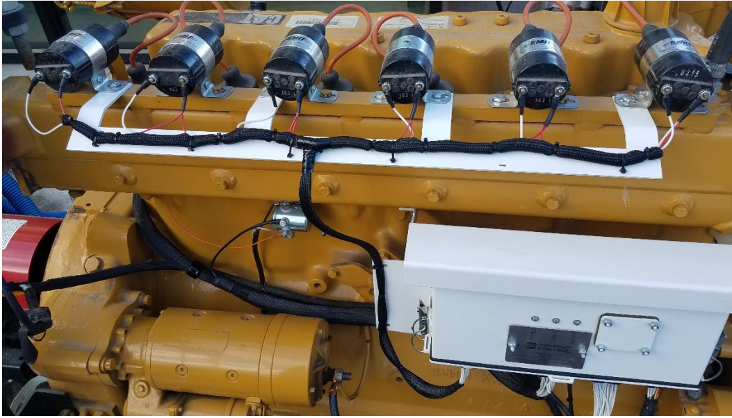
Figure 3. Coil harness attached to bracket
